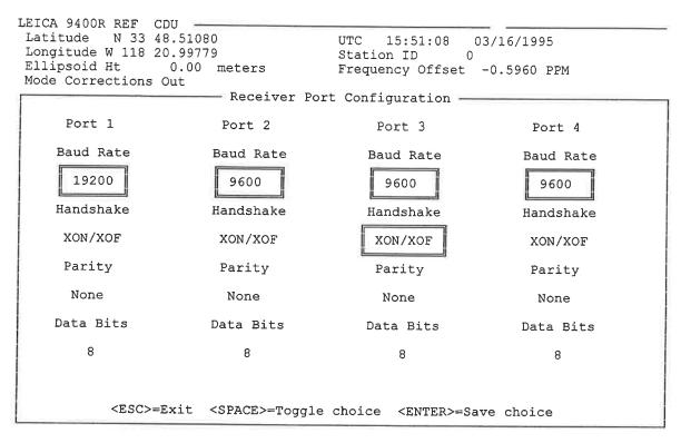
Figure 3-18. Receiver Port Configuration Screen
